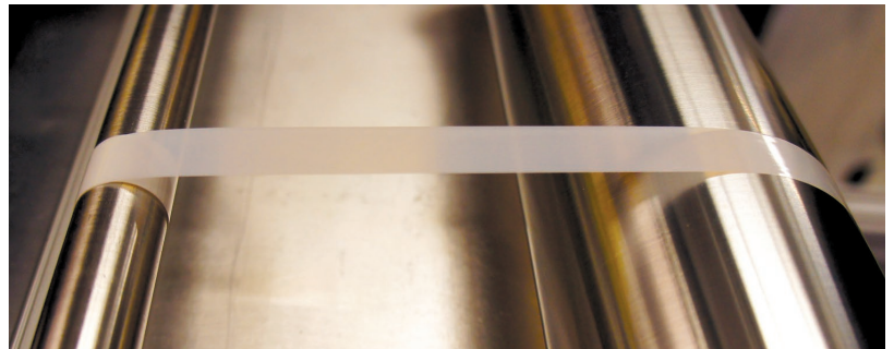
1 cm wide strip of Thin E-Strate ® passing around process equipment rollers
