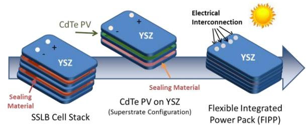
**Figure 7. Flexible Integrated Power Pack (FIPP) combining the SSLB and high efficiency CdTe PV in a single vertically integrated package.**
