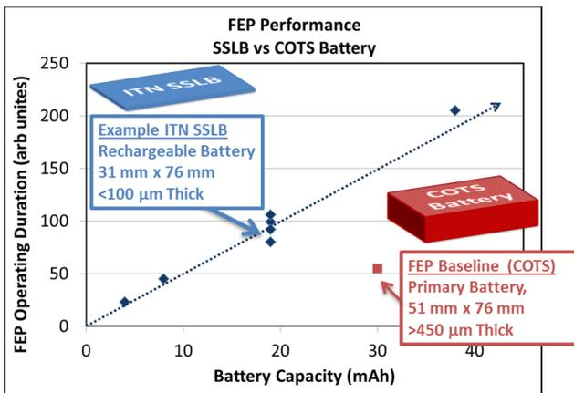
**Figure 6. SSLB achieved over twice the duration with less than one-fourth the size of baseline batteries in powering a flexible electronic device test case chosen in concert with the FlexTech Alliance.**
