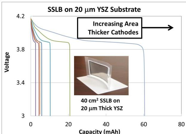
**Figure 3. SSLB cells, deposited on 20 μm thick YSZ, have capacity that increases linearly with area and cathode thickness; inset is a large area SSLB.**
